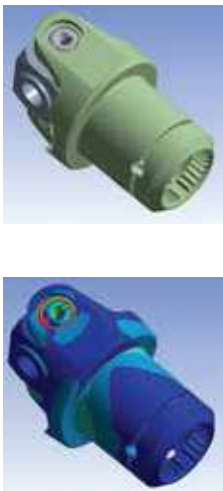
APEX design engineers utilize 3-D solid models and finite element analysis (FEA) to develop and evaluate different design options.
