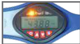
The yellow LED illuminates within 10% of target torque.
